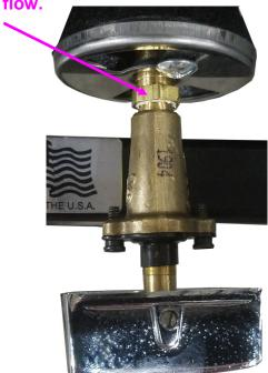
If for some reason a burner does not light, turn the knob to "OFF" and turn off gas source. Wait 5 minutes for gas to dissipate, then restart lighting instructions. **CAUTION: GRIDDLE WILL BE EXTREMELY HOT.**
